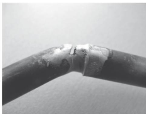
**Fig. 5.** Tube destruction effected by brazing alloy melt
