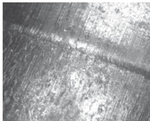
**Fig. 4.** Area of diameter change on a refrigerator tube after reducing
