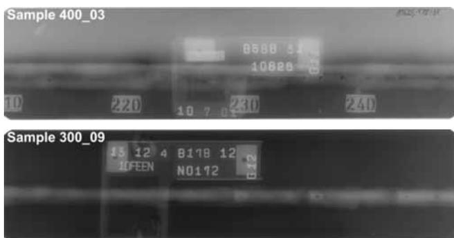
Fig. 2. Exemplary results of radiogram thresholding using optimised processing chain.
