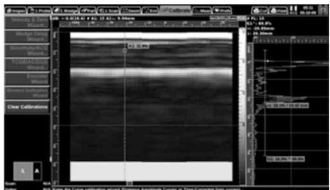
**Fig. 8.** WEWP, 1 MHz, 18.7 mm GFRP
