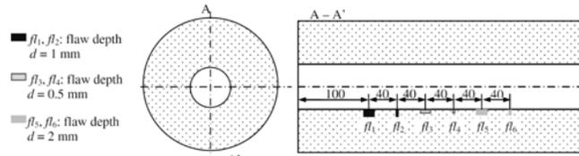
**Fig. 8.** The view with dimensions of the hollow axle sample
