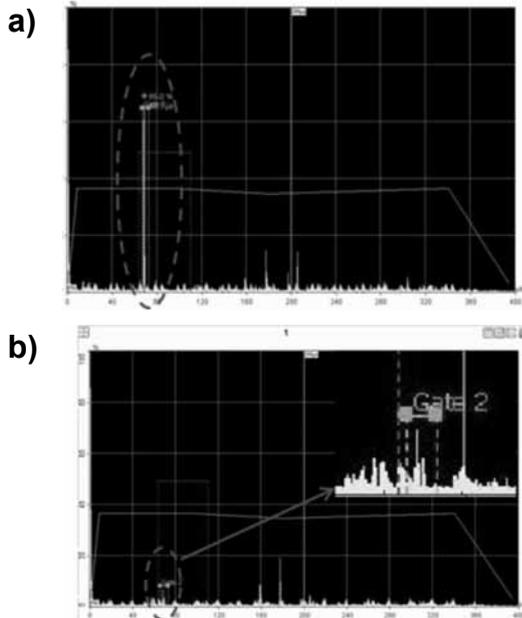
**Fig. 5.** A-scan response using the 45° incidence probes from: a) 3 mm deep notch, b) 1 mm deep notch.
