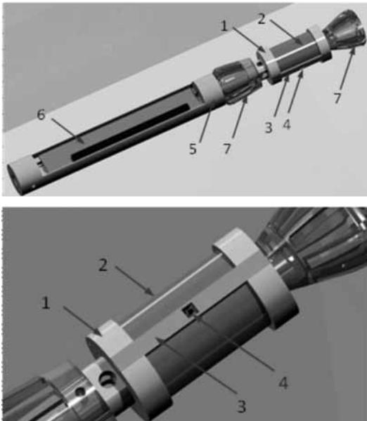
**Fig. 7.** Simplified view of the transducer; 1 – plastic bobbin, 2 – excitation coil, 3 – support plastic element for Hall effect sensors, 4 – 3 x Hall effect sensors, 5 – plastic compartment for electronic boards, 6 – electronic board, 7 – front and rear plastic centering elements
