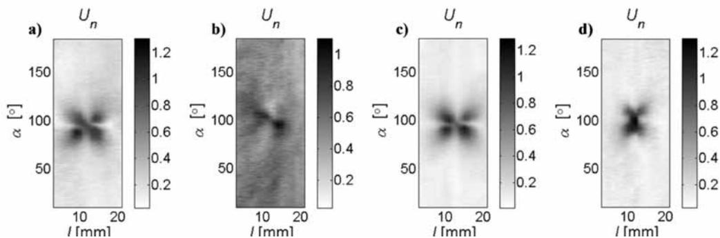
**Fig. 10.** Norm values of the measured x, y and z components signals obtained during 2D scanning of: a) notch no.1 (1 mm depth), b) notch no.3 (0.5 mm depth), c) notch no.5 (2 mm depth), d) notch no.2 (1 mm depth).
