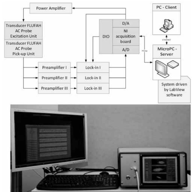
**Fig. 6.** Block scheme and a photo of the electromagnetic subsystem
