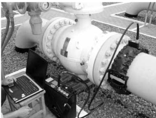
**Fig. 1.** The GWUT components: To the right is an inflatable ring that contains the transducers mounted around the pipe. The ring is connected to the G3 instrument (black, stands on the ground) by a connector cable. From the G3 the information is loaded onto a computer where the analysis is made
