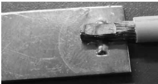
**Fig. 2.** Resistance projection weld on a resistance-compact strand, cross-section area 6 mm<sup>2</sup>
